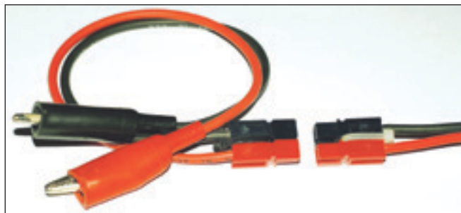
Figure 3 — A pair of disconnected Powerpole connectors. Note that the two connectors are identical, but can be connected together — this is what we mean by genderless connections.
