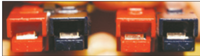
Figure 6 — Standard orientation of Powerpole connectors.
