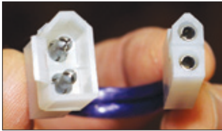
Figure 5 — Comparison of 20 A (on left) and 7 A Molex connectors. While appearing similar, they cannot be connected.
