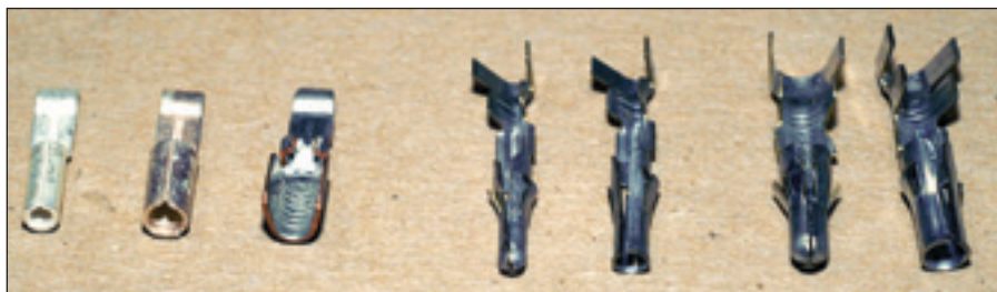
Figure 8 — Comparison of the three sizes of Powerpole pins (left) with the 20 and 7 A Molex pins. Note that all three sizes of Powerpole pins fit in the same size housing and that they can be interconnected.
